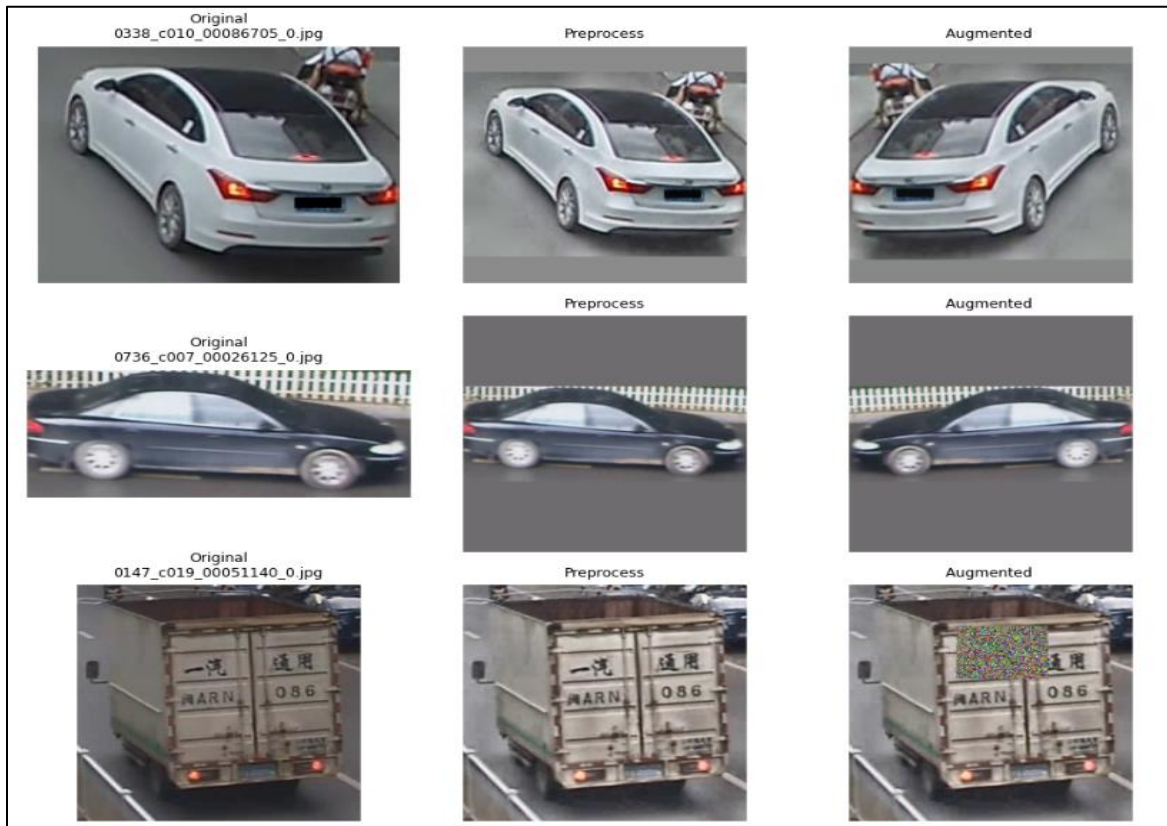
Fig. 2: Comparison between original, preprocessed, and augmented vehicle samples.
